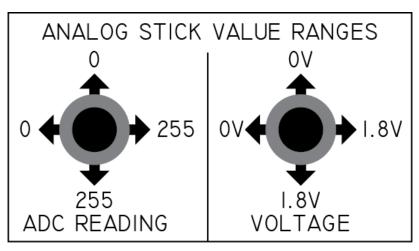
After entering this command you'll be asked to press A without touching any analogs to provide a baseline value. Then, one-by-one, move the sticks and triggers as commanded pressing A to set each value. Try to keep the sticks centered and pressed as far as possible when setting values.
