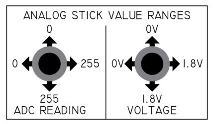
Note the usage of "upper" and "lower" below refers to the numbers used, ie, pushing analog stick left results in a lower number than pushing it right. The analog triggers work in a similar way, the lower number "pulls" the trigger while the higher number is the released state.
